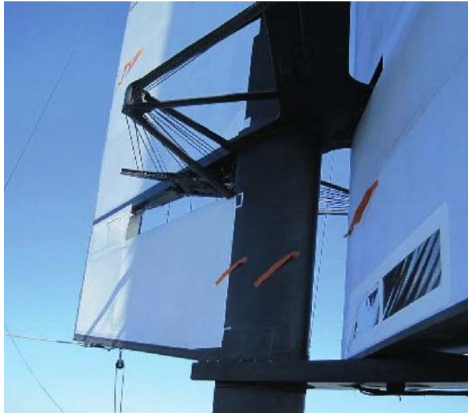
“Winny’s System,” developed by Thiha Wing, adjust the 9 port and 9 starboard aft-flap control lines so they can be trimmed together or independently.
