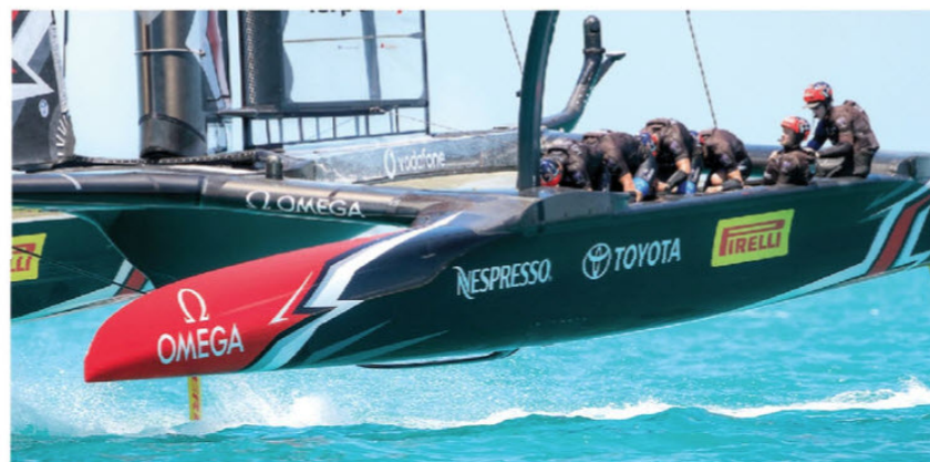
Deceptively smooth – but deadly. A calm-looking Glenn Ashby works the Gameboy, the cyclors pumping away steadily and nicely tucked in to minimise aero-drag. A look that compared dramatically with the flailing arms pressuring the hydraulics onboard Oracle
